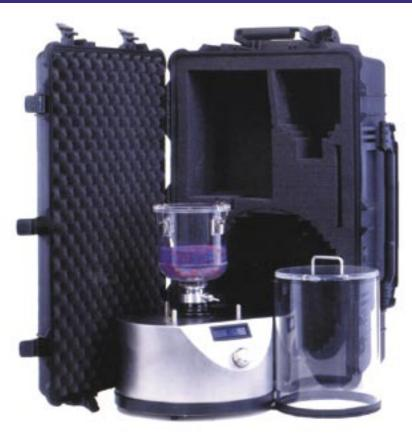
All components fit into the carrying case, which is 33" x 21" x 11."
